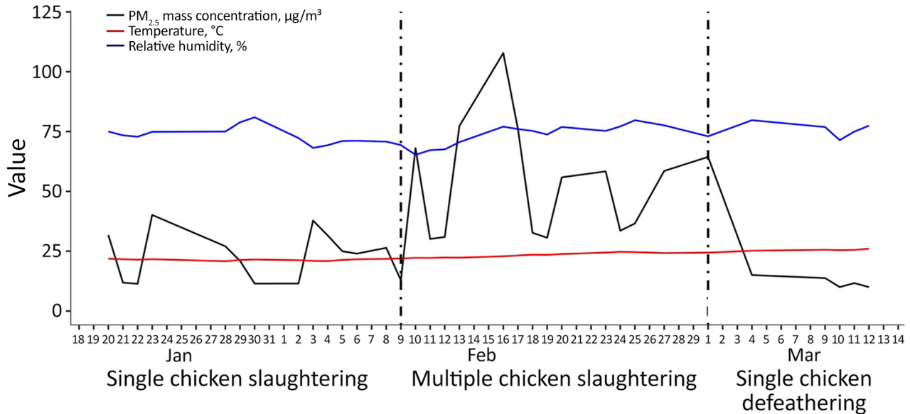
Figure 6. Trend and variability of average particulate matter mass concentration, temperature, and relative humidity in study of respirable aerosol production and reduction of avian influenza transmission risk during chicken processing, Bangladesh Livestock Research Institute, Savar, Dhaka, 2020. Results are shown for single (1 chicken at a time) and multiple (4 chickens at a time) chicken slaughtering events and defeathering events (1 chicken at a time). PM 2.5 , particulate matter <2.5 µm in diameter.
