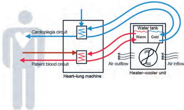
**Figure 1.** Schematic representation of heater–cooler circuits tested for transmission of *Mycobacterium chimaera* during cardiac surgery despite an ultraclean air ventilation system. Blue arrows indicate cold water flow, and red arrows indicate hot water flow and patient blood flow.
